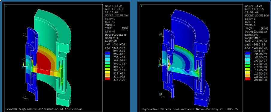
Thermal and mechanical stress analysis were performed for the window under 300 kW RF power using the ANSYS code.
