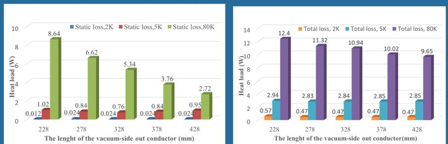
The simulation shows that the heat loads to 2 K flange and 5 K are too high for the Cryostat heat loss controlling. The heat load to 2 K flange and 5 K anchor are mainly consist of the dynamic heat loss, and it could not be minished by extend the vacuum-side out conductor.
