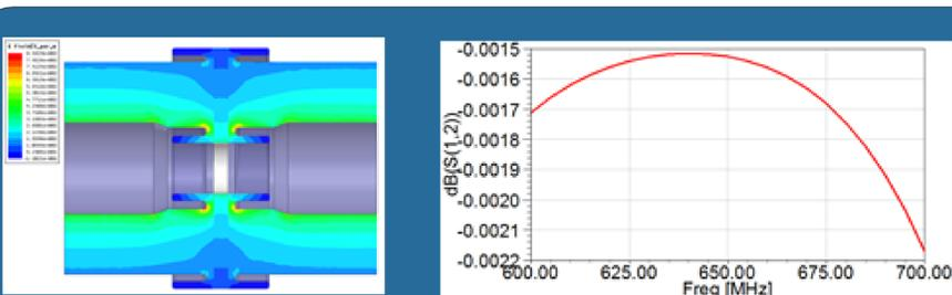
The choke is an impedance-matching structure, meanwhile provides shielding for the window braze joints to reduce the electrical field. As shown in the figures, the electrical field near braze joints is obviously lower because of the choke structure and the window match the impedance well.
