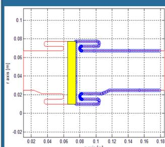
The window (left) and coaxial line (right) geometries for multipacting simulation. The blue dots are initial electrons.
