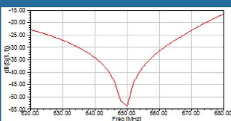
The S11 curve of the integrate coupler. The S11 is smaller than -50 dB at 650 MHz. And the bandwidth is about 40 MHz at S11 = -25 dB.
