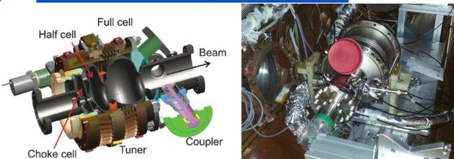
The SRF Photoinjector is a 1.4 cell cavity optimized for high emission phase and peak on-axis longitudinal electric field close to the cathode within the half-cell. The cathode carrier is a demountable, thermally and electrically isolated stalk on which multi-alkali photocathodes will be deposited, similar to the HZDR system for the 3.5-cell SRF gun at ELBE.
