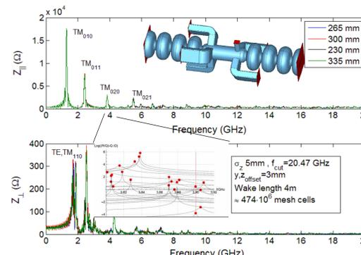
Wake calculation for different connecting beam tube lengths. Coupling at beam harmonics needs to be avoided.
