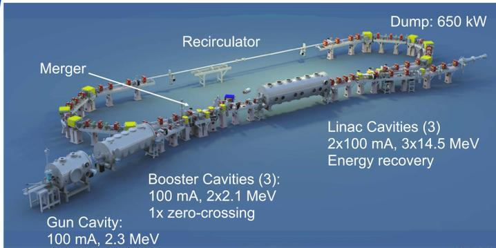
bERLinPro's main goal is the ERL operation of a **low emittance, high current beam** ( $\epsilon_n < 1 \text{ mm mrad}$ ,  $I = 100 \text{ mA}$ ).
