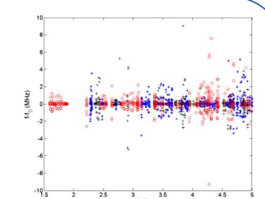
HOM frequency variation due to end-cell tuning for field-flat tuned geometries obtained by perturbation method [14, 16]
