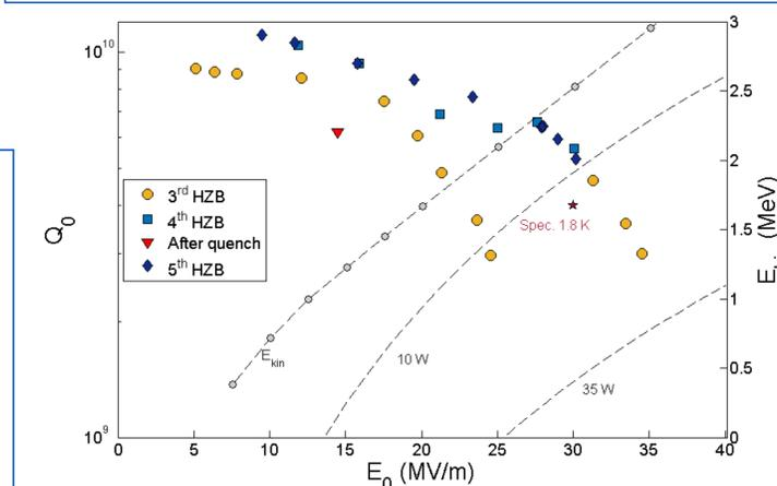
Latest horizontal Q<sub>0</sub> measurements of Gun1.0 at HZB at 1.8 K using critically coupled antennas. For reference the max. energy gain at optimum phase is given.
