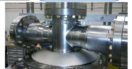
Details of the fundamental power coupler port with the tapered outer conductor tube. This section was mainly modified from the Cornell design
