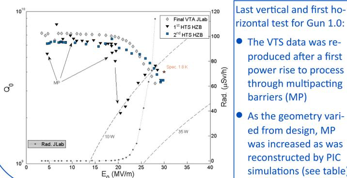
Last vertical and first horizontal test for Gun 1.0:
