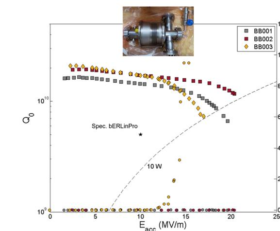
Booster cavity vertical tests at JLab before and after helium vessel welding (except for BB004) at 1.8 K. Due to leakage problems below  $\lambda$  point at the FPC NbTi flanges, cavity BB001 was only measured at 2.0 K.
