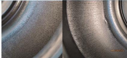
Figure 2: Macrostructures on cavity SPL #1
