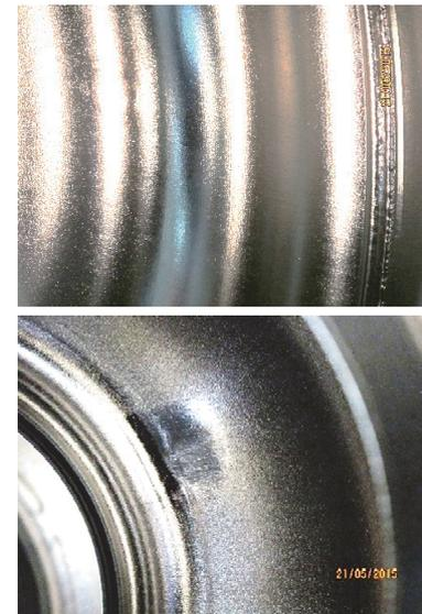
Figure 6: SPL #2 inner surface after the 6th run. Top is the equator and bottom the iris with a noticeable mechanically polished area.
