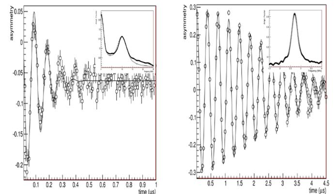
Figure 4 –  $\mu$ SR spectra depicting the mixed state (left) and the normal state (right). The Fourier transforms of the data are inset on the spectra.
