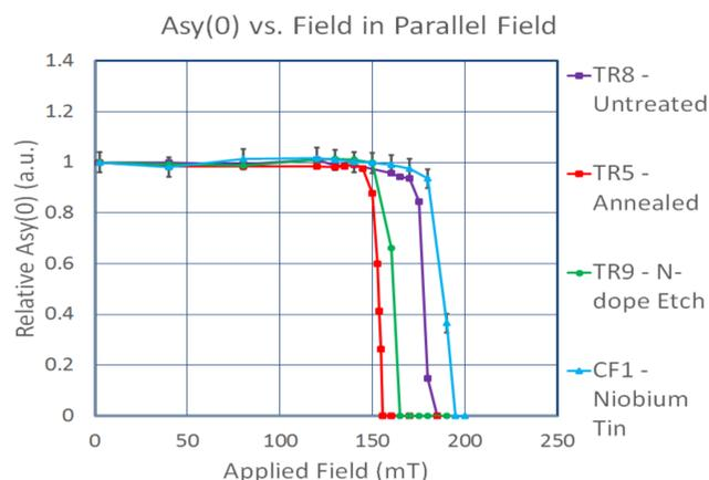
Figure 3 – Plotting "Relative Asy(0) vs. Applied Field" values illustrates the transition from the meissner state to the mixed state in PF.
