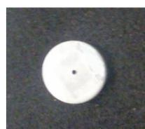
Figure 5 – Sample CF1 (Nb<sub>3</sub>Sn coated Nb).
