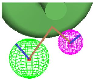
Figure 1: Quench measurement with two OSTs on an elliptical single cell cavity. The red points show the detector positions. Spheres are calculated from literature values of second sound. Note that the spheres do neither intersect nor touch the cavity surface. Desy uses an algorithm that minimizes the distance from the spheres to the cavity surface to find the quench spot (brown lines)
