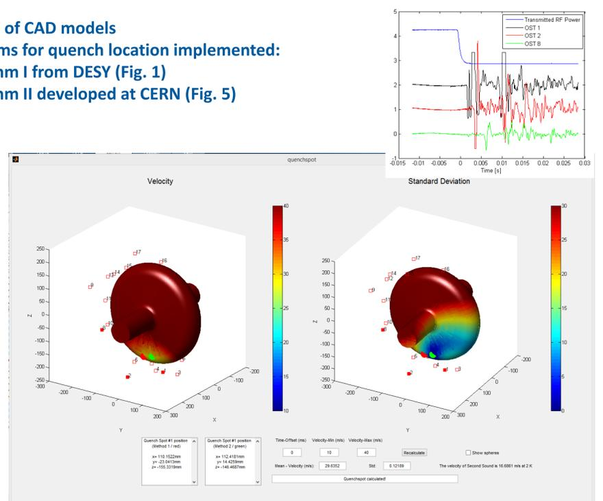
Figure 6: Output window of the quench localisation software. Red/Green dot is the quench spot as predicted by Algorithm I/II. Signals from OST 1,2 and 8 were used for localisation (closed symbols). OST data is shown in upper picture. The slope in the data is consistent with the wider angle between quench spot and detector 8.
