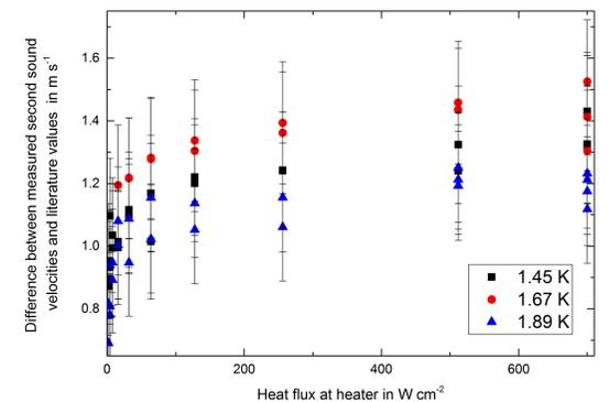
Figure 3: Difference between the measured second sound velocity and the literature data versus applied heating flux densities. Data are shown for one OST at 5 cm distance directly facing the heat source.
