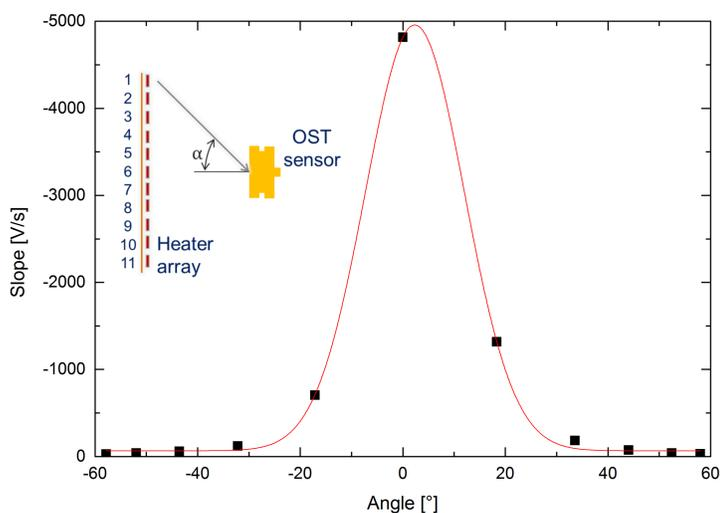
Figure 4: Measured slope of the OST signal dependent on the incident angle to the membrane of the OST. Inset: Schematic of the experimental set-up to test the influence of the inclination angle of the second sound wave on the OST membrane.
