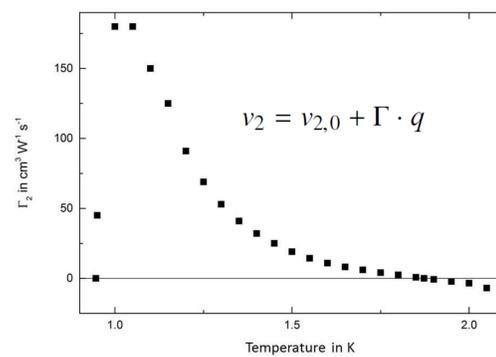
Figure 2: Plot of measurement data of the heat flux amplitude factor  $\Gamma$  by Dessler and Fairbank. Important temperature for our investigation is the change in sign at  $T=1.873$  K
