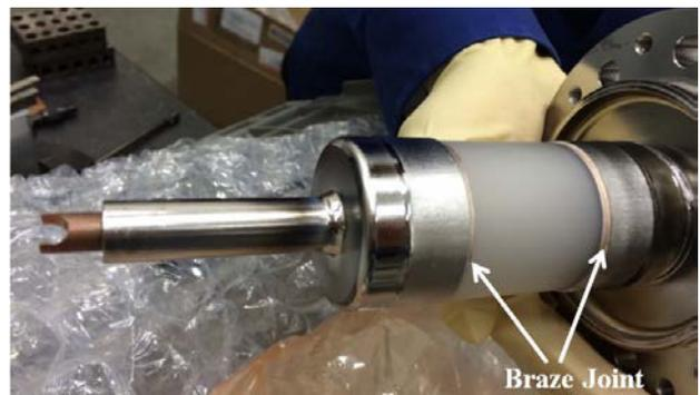
Figure 8: Braze joint at the end of the sapphire window.
