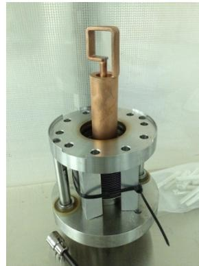
Figure 5: The Fundamental Power Coupler.
