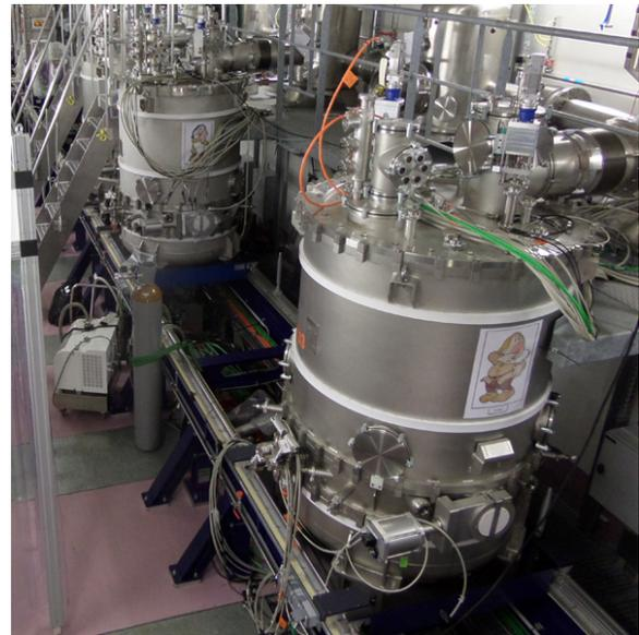
Figure 11: High beta cryomodules installed on LINAC.
