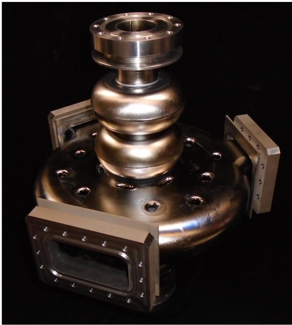
Figure 3: The 5-cell cavity for high gradient testing, made from bulk niobium.
