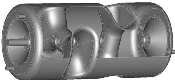
Figure 1: 325 MHz,  $\beta_0 = 1$  double-spoke cavity.
