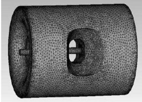
Figure 5: 325 MHz,  $\beta_0 = 1$  single-spoke cavity.
