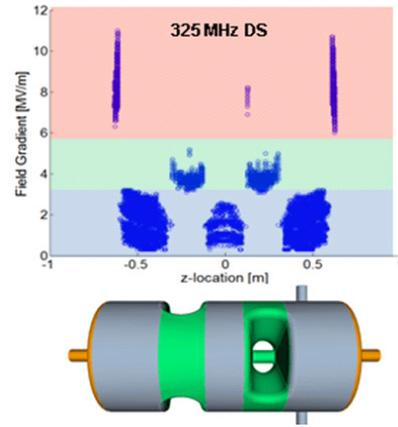
Figure 6: Multipacting simulations for a 325 MHz,  $\beta_0 = 1$  double-spoke cavity. Multipacting activity is shown for increasing accelerating gradient in terms of the longitudinal position along the cavity.
