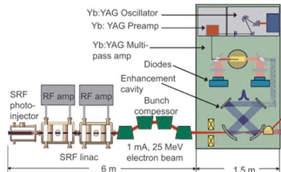
Figure 4: Conceptual layout of an inverse Compton source.
