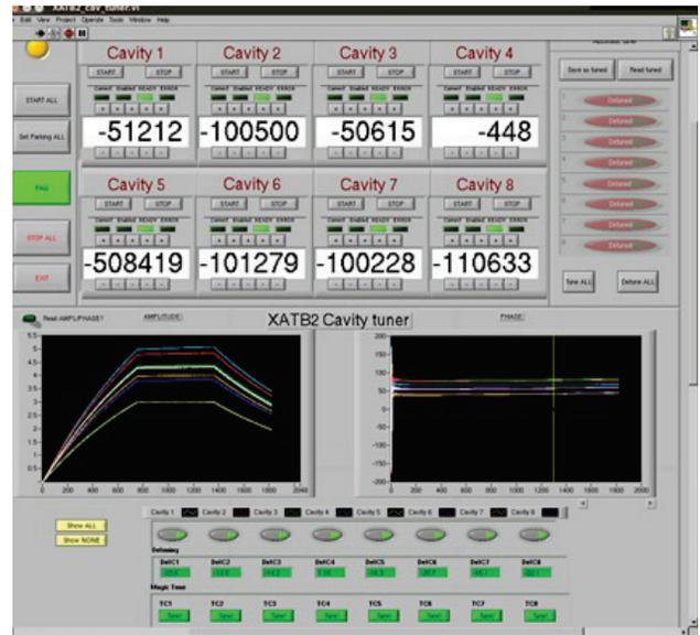
Figure 8: Cavities tuning software for low gradients.
