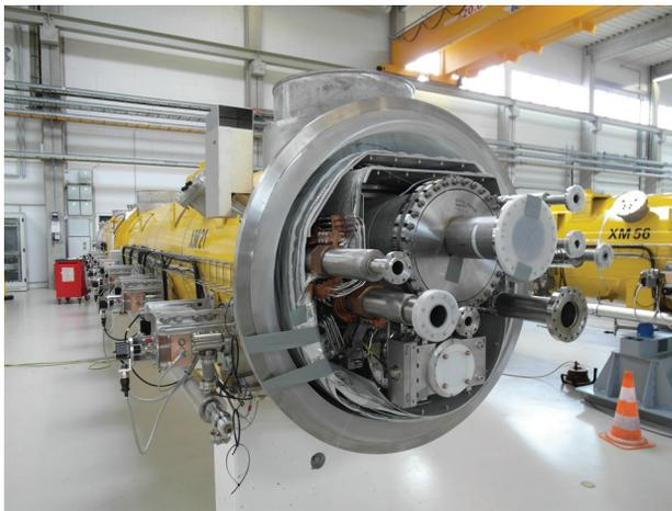
Figure 2: GRP adapter already installed on the cryomodule.
