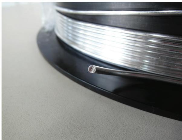
Figure 3: 3.5 mm diameter indium seal.
