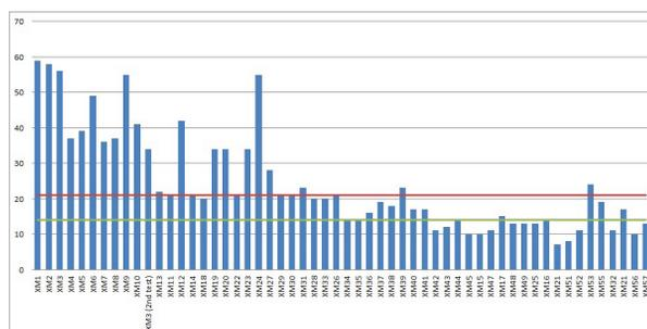
Figure 6: Number of days inside the test bench for each tested cryomodule. Red line is 21 days. Green line is 14 days.
