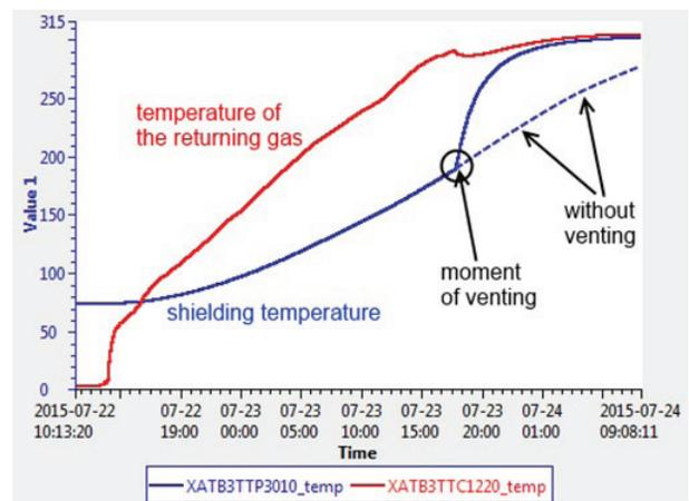
Figure 5: Impact of the insulation vacuum venting to warm - up procedure.
