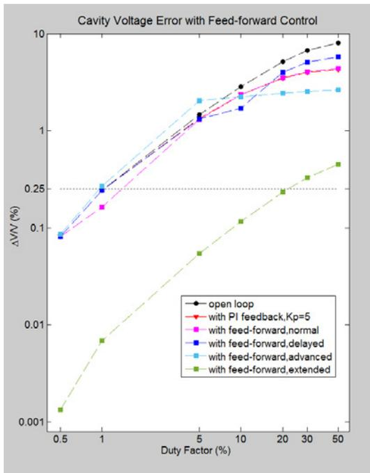
Figure 5: Cavity voltage errors with additional feed-forward control and different timing modes.
