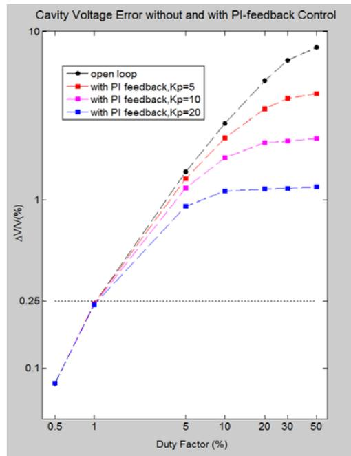
Figure 4: Cavity voltage errors with different PI controller gain values. Dashed horizontal line indicates voltage error control requirement.
