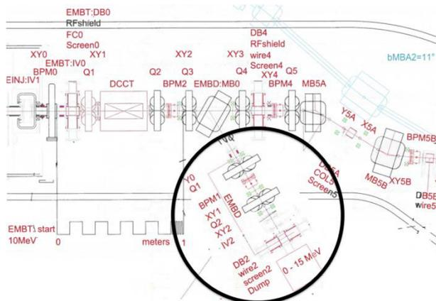
Figure 6: EMBT section of e-linac. Location of beam dump diagnostics are shown in black circle.
