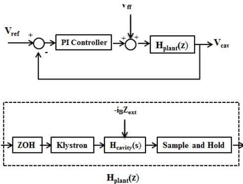
Figure 3: Above: Feedback and feedforward block diagram. Below: Discretized model of beam-loaded cavity and klystron.
