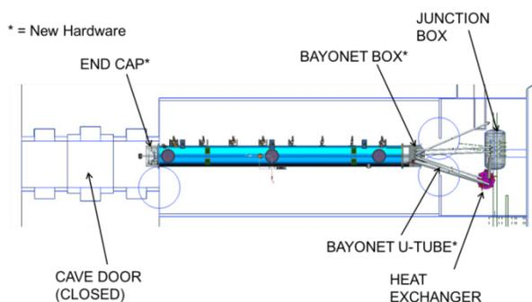
Figure 3: CMTF Layout of CM with U-tubes and HX.
