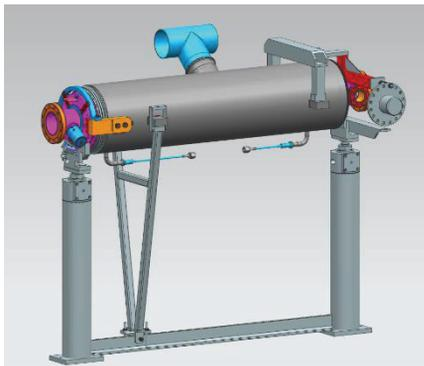
Figure 3: LCLS-II dressed cavity installed on the cleanroom assembly fixture.
