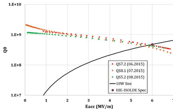
Figure 6: Q0 (Eacc) at 4.5K performance for the CM2 cavities.
