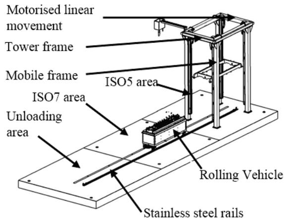
Figure 4: Cleanroom tooling.
