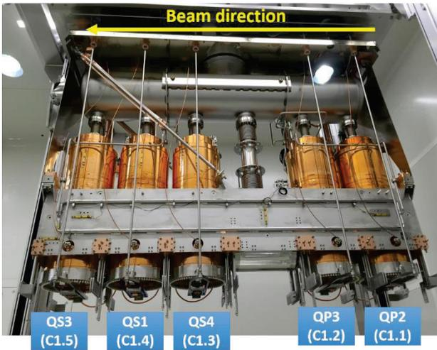
Figure 5: Cavities installed on CM1.
