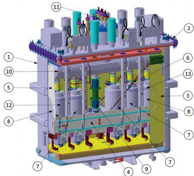
Figure 1: The complete HIE-ISOLDE high- $\beta$  cryo-module; 1 Vacuum vessel lower box, 2 Vacuum vessel top plate assembly, 3 Thermal shield lower box, 4 Support frame, 5 Suspension end plate, 6 Tie-rod, 7 Inboard cavity, 8 Outboard cavity, 9 Down tube to solenoid, 10 Helium vessel, 11 Chimney assembly, 12 Support frame cooling supply, 13 Support frame cooling return, 14 Mathilde targets, 15 Mathilde viewport.
