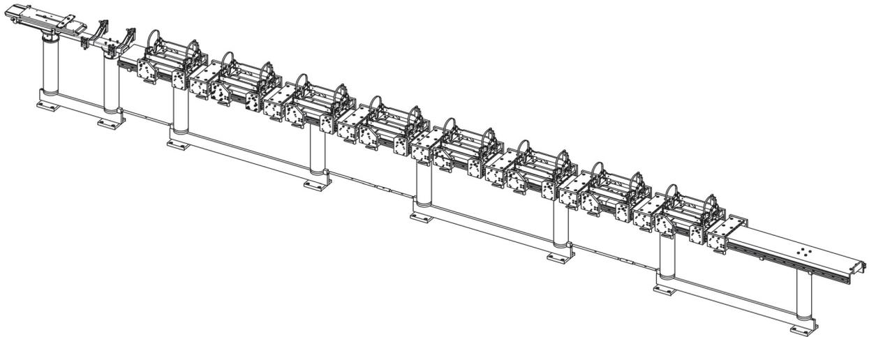
Figure 8: 3-D drawing of the assembly platform for eight 3.9 GHz resonators with alternating power coupler orientation.
