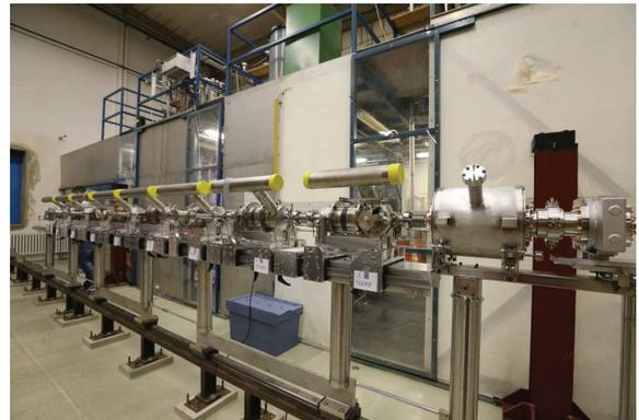
Figure 9: 3.9 GHz string with BQU on right hand side completed.
