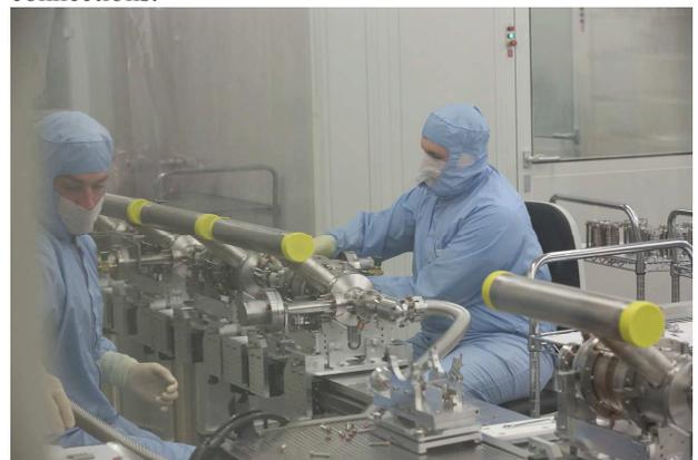
Figure 7: Assembly of cavity 3.9 GHz string for Module No.: X3M1.
