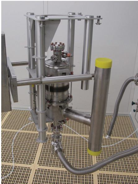
Figure 2: 3.9 GHz cavity dressed with helium tank in frame during leak check.
