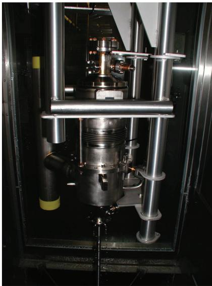
Figure 4: dressed 3.9 GHz cavity during HPR.
