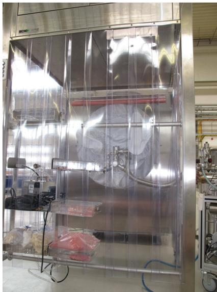
Figure 3: Local cleanroom at AMTF hall for dismantling the vacuum diagnostic stars.
