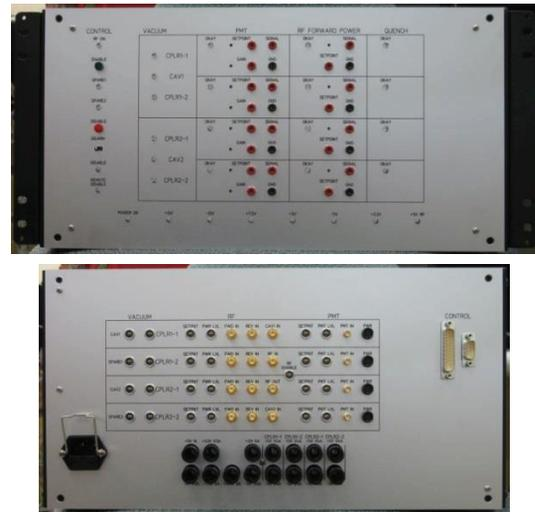
Figure 9: Front (top) and rare (bottom) panels of interlock box.
