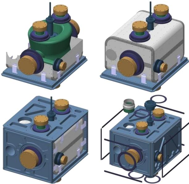
Figure 5: Assembly of DQW shield and helium vessel.
