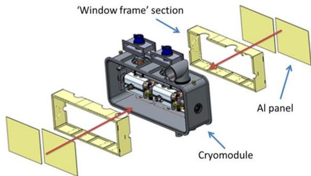
Figure 9: Thermal shield assembly.
