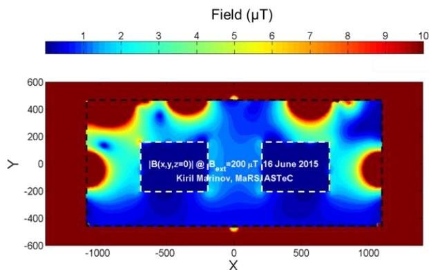
Figure 3: OPERA shielding analysis.
