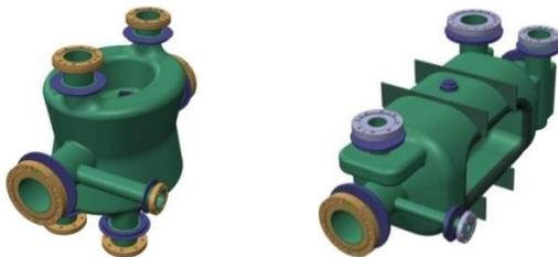
Figure 1: DQW (left) and RFD (right) prototype crab cavity models.
