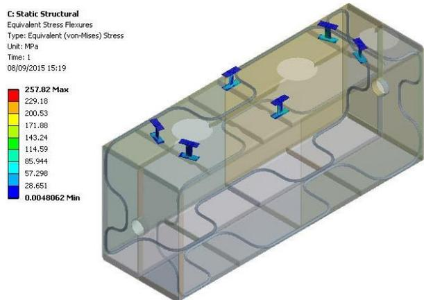
Figure 8: Cool down stress on flexure mounts.
