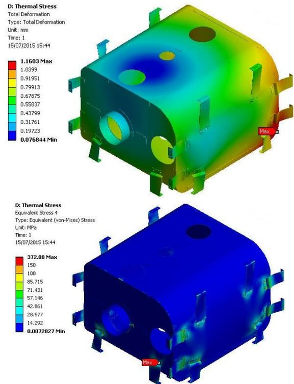
Figure 6: Thermal deformation (top) and stress (bottom) of DQW magnetic shield at 2 K.
