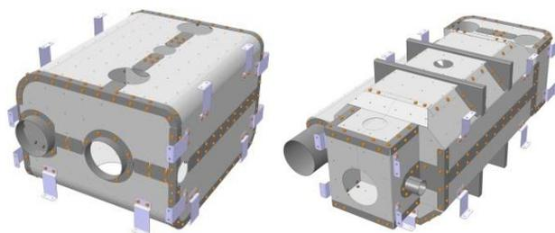
Figure 4: cold magnetic shields DQW (left) and RFD (right).
