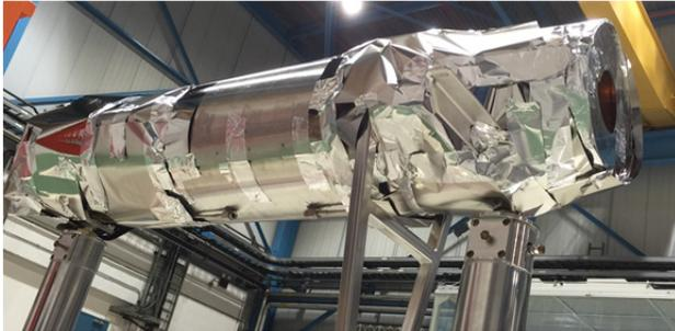
Figure 5: A dressed 9-cell cavity covered with local magnetic shield and augmented with magnetic foils.
