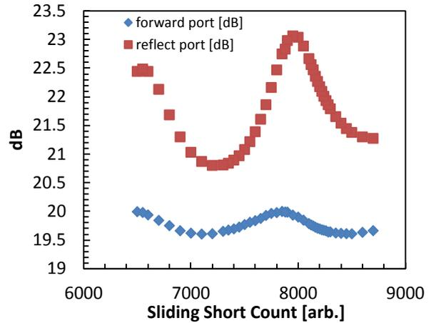
Figure 6: A non calibrated relative measurement of port coupling for a Narda® directional coupler.
