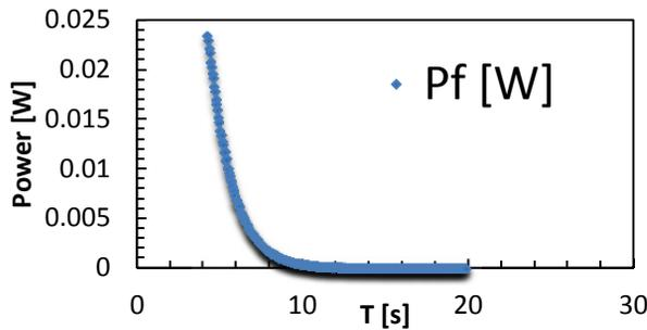
Figure 5: A forward power trace measured for a LCLS-II 9-cell cavity horizontal test.
