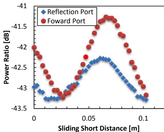
Figure 4: A measured coupling factor variation for a 40dB directional coupler (Courtesy of M. Middendorf).
