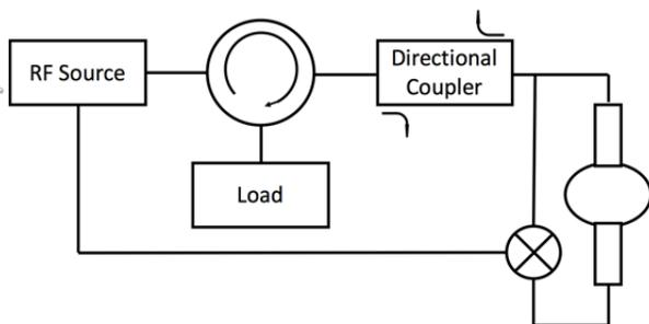
Figure 1: A dramatically simplified cavity test diagram.
