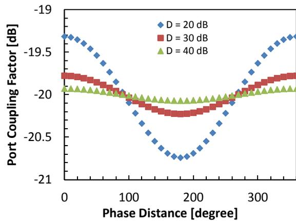
Figure 3: Calculated coupling factor variation of a 20dB directional coupler with different directivity (D).
