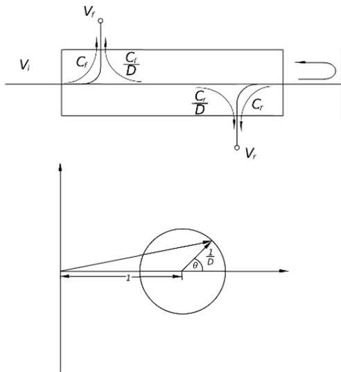
Figure 2: Voltage measured at one of the coupling port of a directional coupler.
