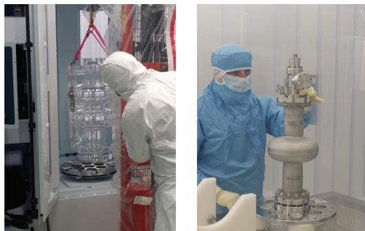
(a) HPR test of transparent cavity model
