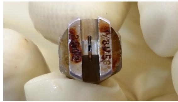
Figure 10: Image of the corroded HPR nozzle.
