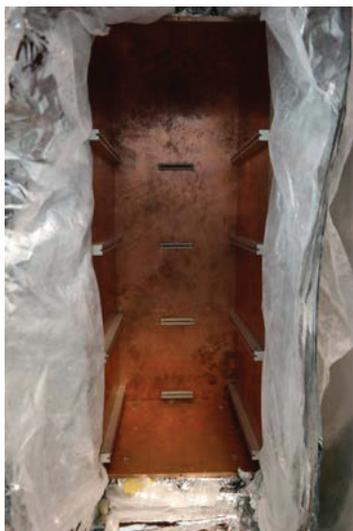
Figure 2: RRR test stand Cu sample measurement box with Al shield and super insulation open exposing with front panel removed.
