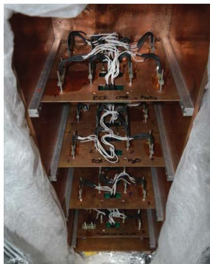
Figure 3: Four small sample boards installed in the Cu box.
