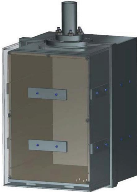
Figure 7: The new test stand test fixture with one of the sides of the shroud and Cu box rendered transparent.
