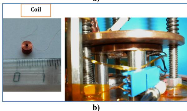
Figure 2: a) Schematic of the local magnetometry facility at Saclay, b) Details of the coil and sample holder.
