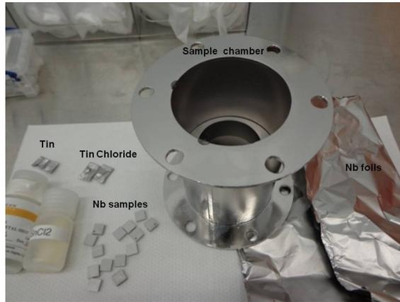
Figure 1: Sample chamber, samples, tin and tin chloride packages, and niobium foils before set up.
