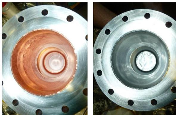
Figure 7: Cu cavity before (left) and after (right) coating.
