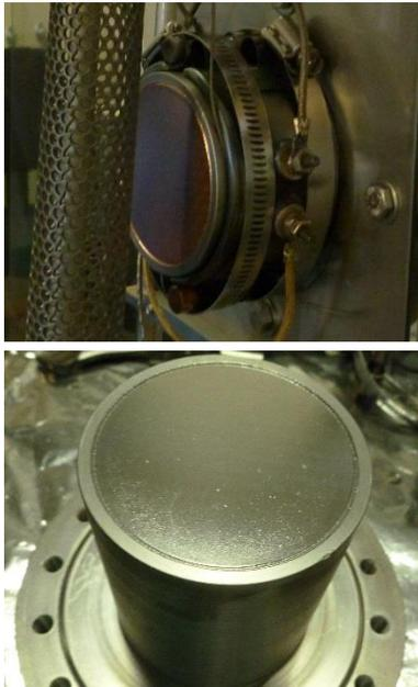
Figure 9: Upper: Resonator mounted for coating. Lower: Coated Resonator.
