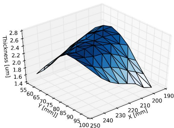
Figure 10: Thickness variation of Nb film on CERN Quadrupole Resonator.
