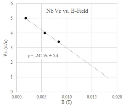
Figure 4:  $V_z$  as a function of magnetic field for the niobium cathode. Blue circles are data points and red squares are an extrapolation.
