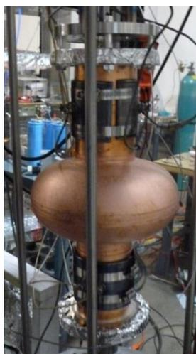
Figure 6: Fermilab cavity mounted with heaters.
