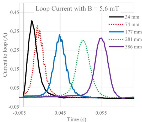
Figure 3: Scan showing ion current to all loops for B = 5.6 mT. Legend indicates the axial location of each loop with respect to the trigger.
