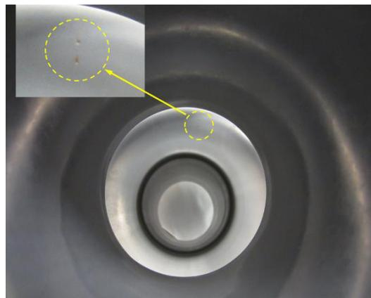
Figure 8: Spots delaminated from high pressure rinse.
