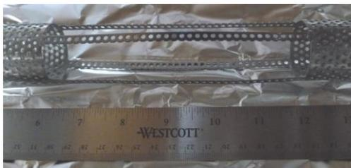
Figure 5: Anode mesh with >90% open area in elliptical region and 33% transmission in the beam tubes.
