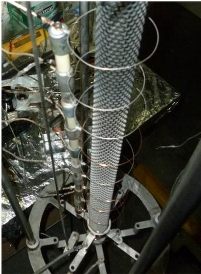
Figure 2: CED electrodes with copper wire loops arranged along the axis to measure spoke axial speed via time-of-flight.
