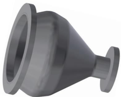
Figure 2: A CAD representation of the Sample Host Cavity, shown without sample plate. During testing, the plate is affixed to the wide opening (“mouth”) of the cavity with a 20/1000” indium seal.
