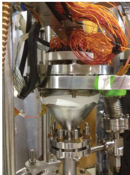
Figure 1: Third-generation Cornell TE sample host cavity with temperature map and external temperature sensors installed.
