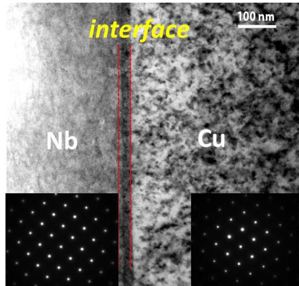
Figure 2: FIB-TEM cross section of a hetero-epitaxial film grown at 184 eV and 64 eV, at 360 °C on large grain Cu.
