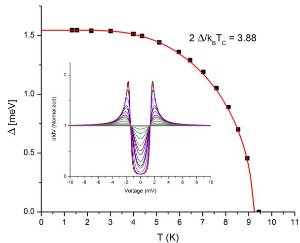
Figure 4: superconducting gap measurement by PCT for the hetero-epitaxial film from Fig. 2.
