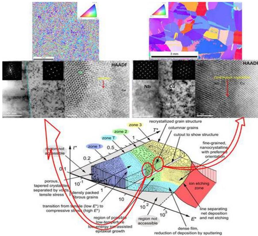
Figure 1: Illustration of the ECR Nb film microstructure variation with the generalized Structure Zone Diagram from [10].
