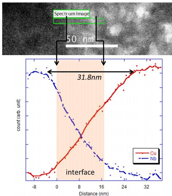
Figure 3: EELS analysis of the Nb-Cu interface of the ECR Nb film from Fig. 2
