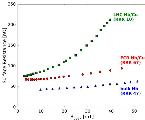
Figure 5: RF Measurement at 400 MHz and at 4 K of an ECR Nb/Cu film compared to sputtered and bulk Nb cavities.
