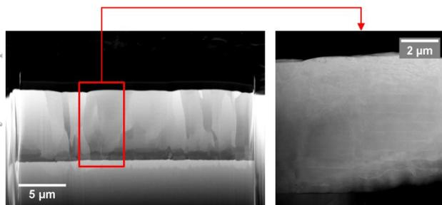
Figure 1: FIB-SEM cross section image of HIE-ISOLDE coating at the middle of the antenna (left) and corresponding High Angle Annular Dark Field (HAADF) TEM image showing the 15 successive layers deposited (right).
