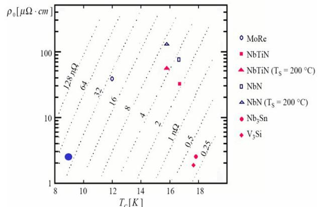
Figure 8: Lines of equal BCS surface resistance in  $(\rho_s, T_c)$  space for different SC materials, adapted from [17].
