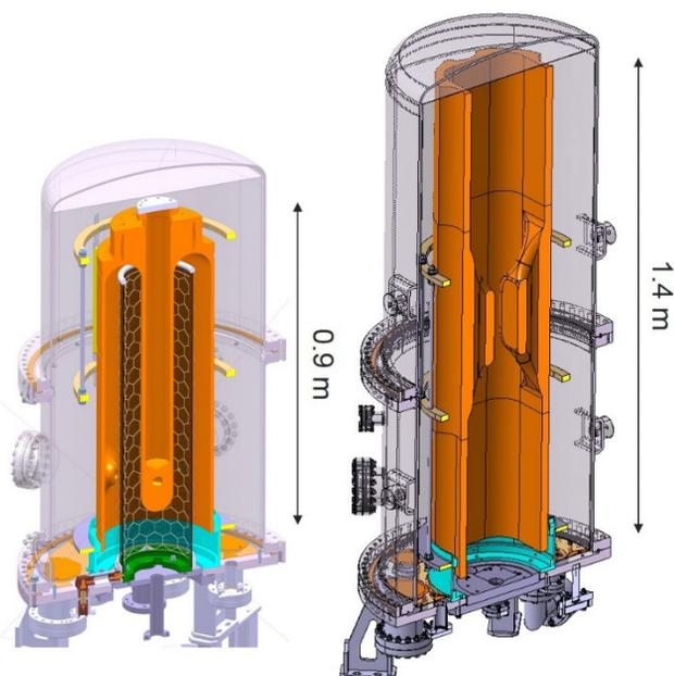
Figure 5: QWR (with single cathode and grids, left) and WOW (right) coating setups.
