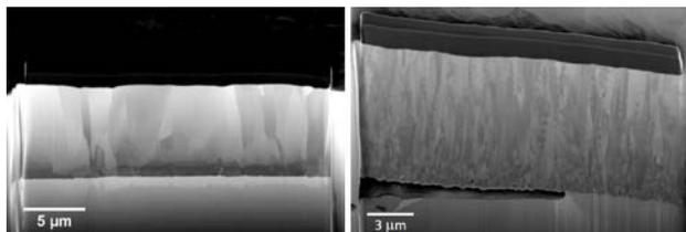
Figure 4: FIB-SEM cross section images of HIE-ISOLDE coating at the middle of the antenna with -80V bias (left) and -120V bias (right) showing the delamination of the layer.
