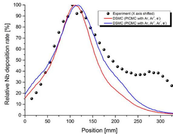
Figure 7: Relative experimental and simulated Nb deposition rate profile along the substrate facing the cathode (DC-magnetron sputtering, 0.01 mbar).
