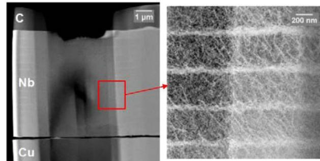
Figure 2: STEM HAADF images show (left) overview of TEM lamella (right) layers 5 to 7 from Cu-Nb interface and gradient of dislocations in between these layers.
