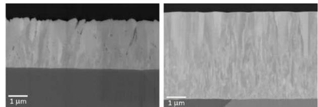
Figure 3: FIB-SEM cross section images of HIE-ISOLDE coating at the top of the cavity with -80V bias (left) and -120V bias + wide cathode (right) showing the densification of the layer.
