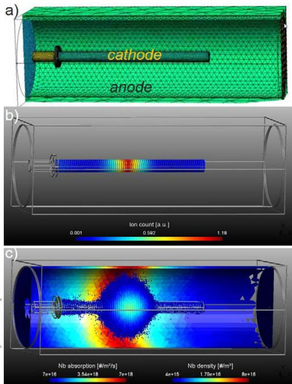
Figure 6: Experimental setup and mesh a), accumulated Ar<sup>+</sup> ion flux onto the cathode during PIC-MC plasma simulation b) and resulting DSMC transport simulation, where Nb is sputtered from the target with a distribution according to the ion bombardment profile c) (DC-magnetron sputtering, 0.01 mbar).
