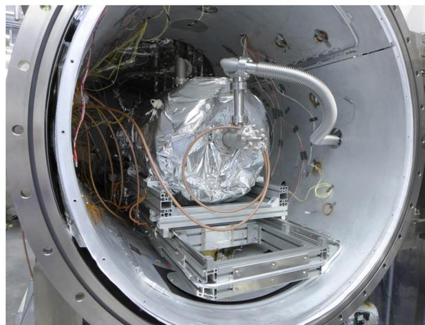
Figure 5: Double-spoke cavity installed in HNOSS.
