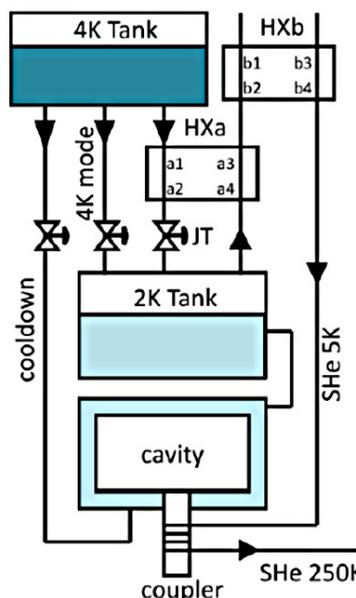
Figure 3: The HNOSS cryogenic circuit.
