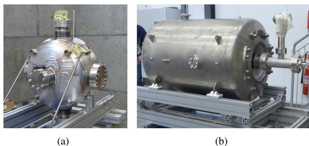
Figure 6: a) The single spoke cavity Hélène and b) the double spoke Germaine from IPN Orsay.
