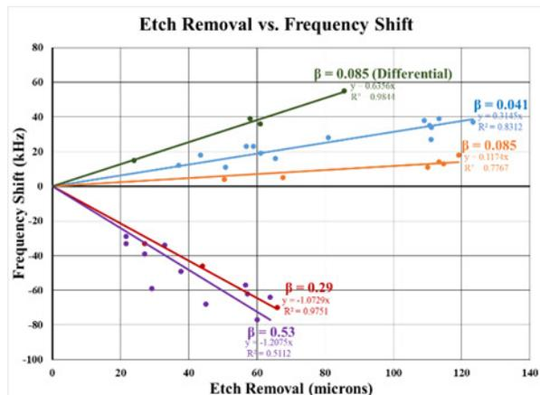
Figure 3: Etch removal versus frequency shift for each FRIB cavity type [4].
