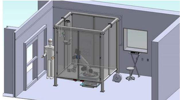
Figure 6: Layout of HPR cell in cleanroom.
