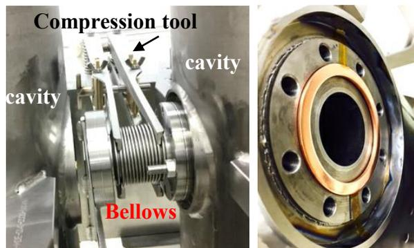
Figure 10: Bellows compression tool (left) and low profile flange with secured copper gasket (right).
