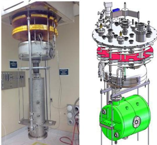
Figure 8: FRIB production insert design.
