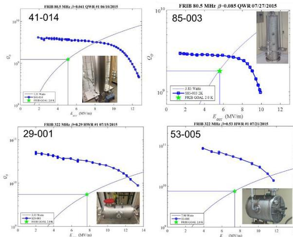
Figure 11: Q<sub>0</sub> vs. E<sub>a</sub> for each FRIB cavity type.
