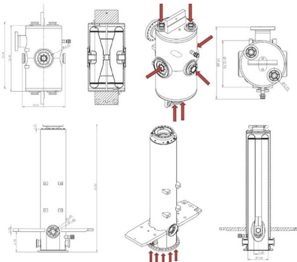
Figure 5: Cleaning access for HWR and QWR.
