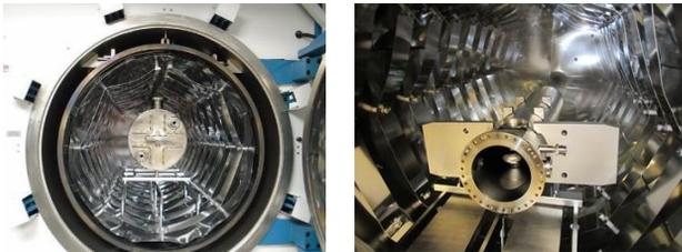
Figure 4: HWR and QWR installed into furnace.
