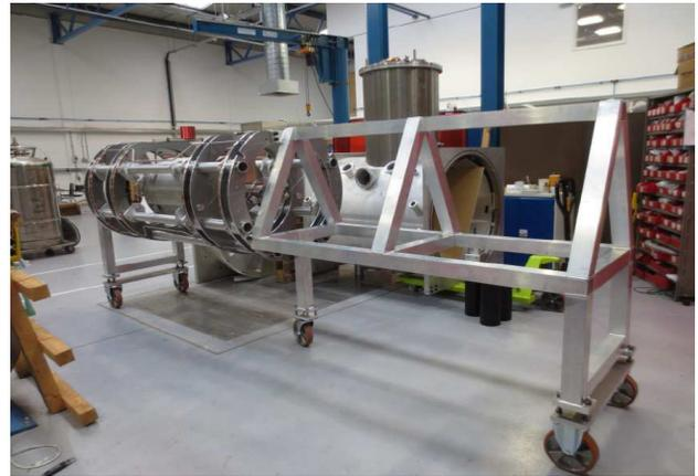
Figure 3: Loading/unloading the cryostat with an aluminum frame.
