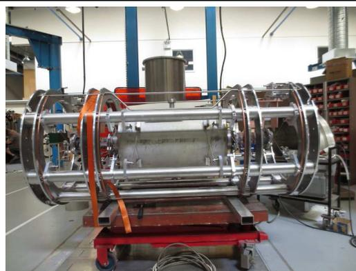
Figure 1: The cw Demonstrator comprising, a CH-cavity embedded by two solenoids supported by a frame, inside the cryostat.
