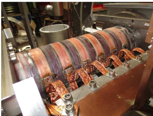
Figure 5: Dry cooled solenoids.
