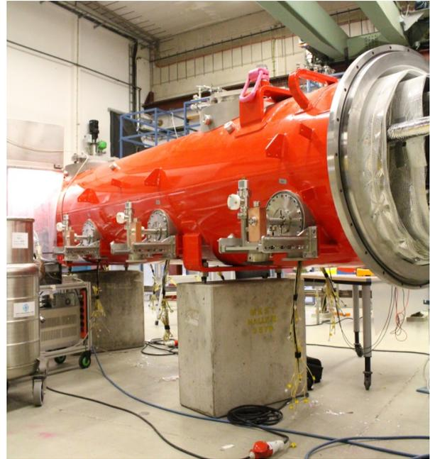
Figure 6: The X3M1 during Warm Coupler parts installation.
