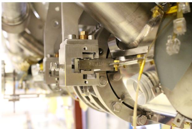
Figure 3: The cavity spring-loaded, roller bearing suspension system.
