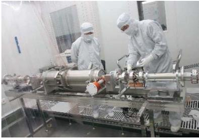
Figure 3: Cavity beamline assembly in clean room.
