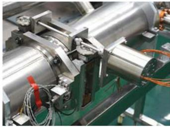
Figure 4: Tuner and piezo.
