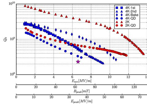
Figure 4: Measurement of Q-value of quarter wave resonator.
