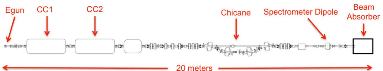
Figure 2: FAST Injector Layout.
