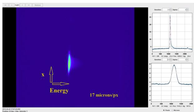
Figure 4: YAG image of first 20 MeV electrons in FAST. The detector is located between the spectrometer magnet and beam absorber.
