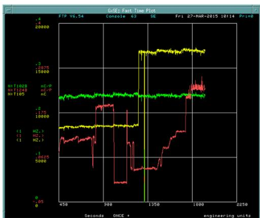
Figure 3: Toroids along the FAST 50 MeV beam line recording first electrons to the beam absorber. The red trace is T124B located immediately after the spectrometer magnet. Measured beam current is  $\sim 0.2$  nCoulombs.
