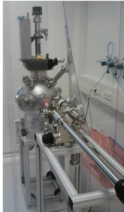
Figure 10: Photograph of the new preparation system for GaAs photocathodes.
