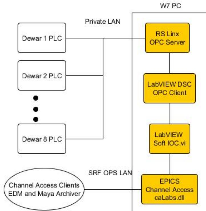
Figure 5: VTA controls, software layers.
