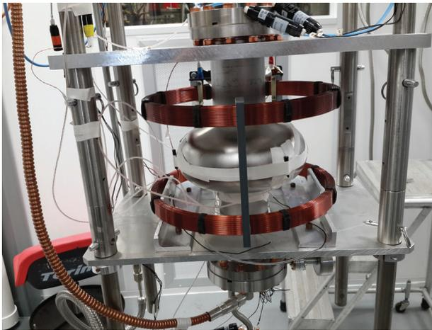
Figure 4: Helmholtz coils for creating axial external magnetic field for vertical test of a 1.3GHz single cell cavity in a typical vertical test orientation of the cavity.
