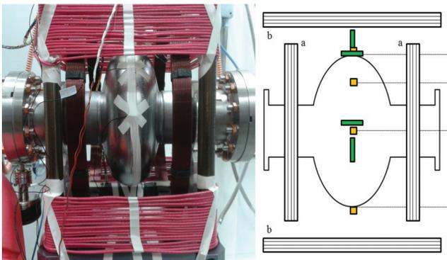
Figure 5: Left: vertical test setup in the horizontal cavity orientation with two pairs of Helmholtz coils, fluxgate magnetometers, and Cernox temperature sensors. Right: schematics of the vertical test setup. Coils for producing cavity axial and cavity transverse fields are labelled a and b respectively. Fluxgate magnetometers are shown as green rectangles. Cernox temperature sensors are shown as yellow boxes.
