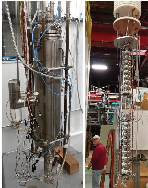
Figure 6: Left: LCLS-II dressed cavity with internal instrumentation and higher order mode couplers installed on the dewar insert at the staging area in preparation for installation into the VTS-2 dewar. Right: two bare 9-cell 1.3GHz cavities on the insert before installation into VTS-1 dewar.
