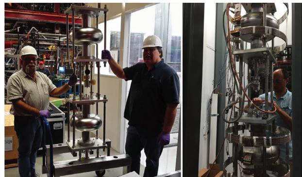
Figure 7: Left: two 650MHz  $\beta=0.61$  single cell cavities in support frame on the cart. Right: two 650MHz  $\beta=0.9$  single cell cavities are being instrumented in vertical test staging area.
