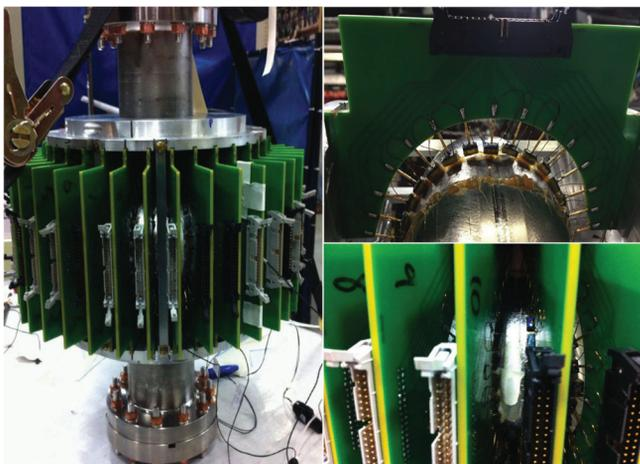
Figure 3: Left: T-map system on 1.3GHz single cell cavity. Top right: single board with resistors along the cavity. Bottom right: view of adjacent boards installed along the equator.
