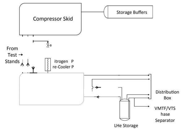
Figure 1: Simplified block diagram of the helium plant.
