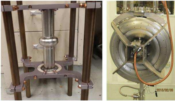
Figure 8: Left: 3.9GHz single cell cavity on a newly fabricated VTS support structure. Right: bare 325MHz single spoke cavity on the insert in the staging area with RF connections for vertical test.
