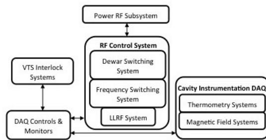
Figure 2: VCTF Control and DAQ system.
