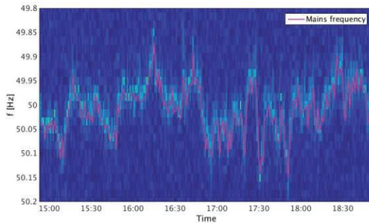
Figure 3: Observation of mains frequency on the beam spectrum.
