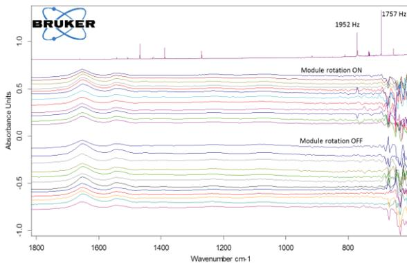
Figure 11: Beam motion spectrum (top) and beamline IR spectra with (middle) and without (bottom) module rotation enabled.
