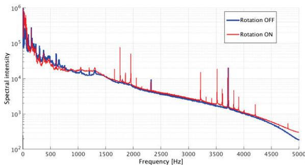
Figure 8: Spectrum of horizontal motion in beam with (red) and without (blue) module rotation.
