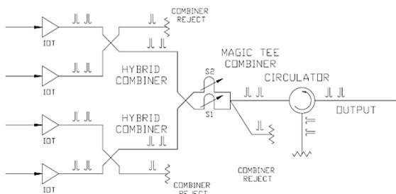
Figure 1: IOT combination scheme used in each of the Diamond 300 kW amplifiers.
