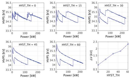
Figure 10: HVPS voltage as a function of output power for different values of *HYST\_TH*.
