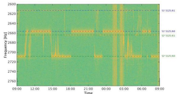
Figure 6: Intensity jumps in horizontal spectrum corresponding to changes in the number of active modules.
