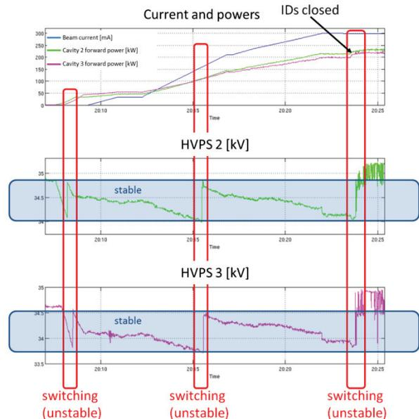
Figure 9: Amplifier power and HVPS voltage during the fill of the storage ring.
