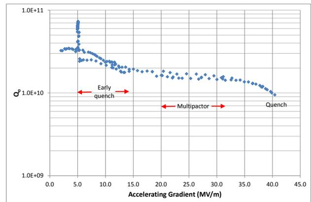
Figure 2: Performance results for PIPSS #03 tested at Fermilab after CBP and a 120°C vacuum bake.
