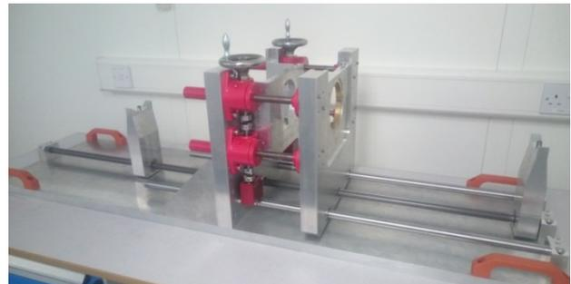
Figure 8: Mechanical cavity tuning fixture.
