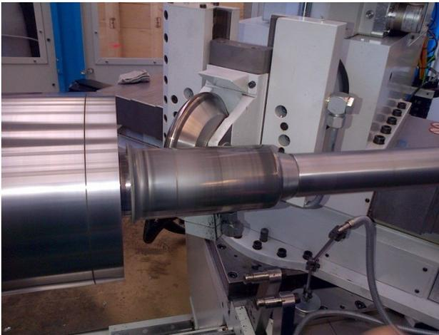
Figure 3: Niobium beam-pipe spinning.
