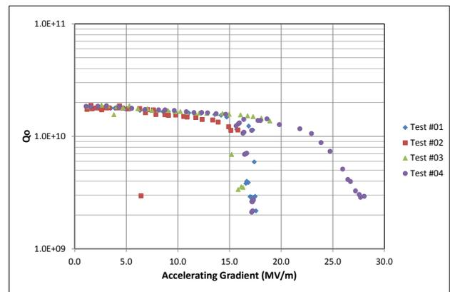
Figure 1: Performance results for PIPSS cavity #01 tested in the vertical test stand at Jefferson Laboratory after BCP processing.
