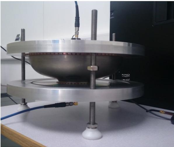
Figure 6: S21 frequency measurement of a half-cell.
