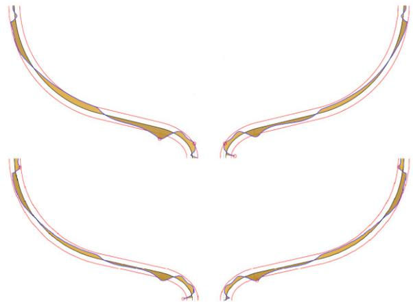
Figure 5: CMM profile of niobium half-cells.
