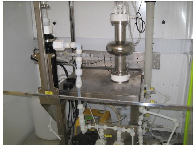
Figure 7: Buffer Chemical Polishing cabinet.
