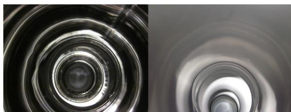
Figure 4: BL1 before and after Nb<sub>3</sub>Sn coating. The cavity received mirror finish CBP, 800 °C x 2 hours, and 5 μm EP before the coating; note the shining appearance of polished niobium[left]. After the coating, the surface is matte gray characteristic of Nb<sub>3</sub>Sn[right].
