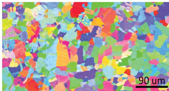
Figure 3: EBSD map of the ECR Nb/Cu coating. The average grain size is about 50  $\mu\text{m}$ .
