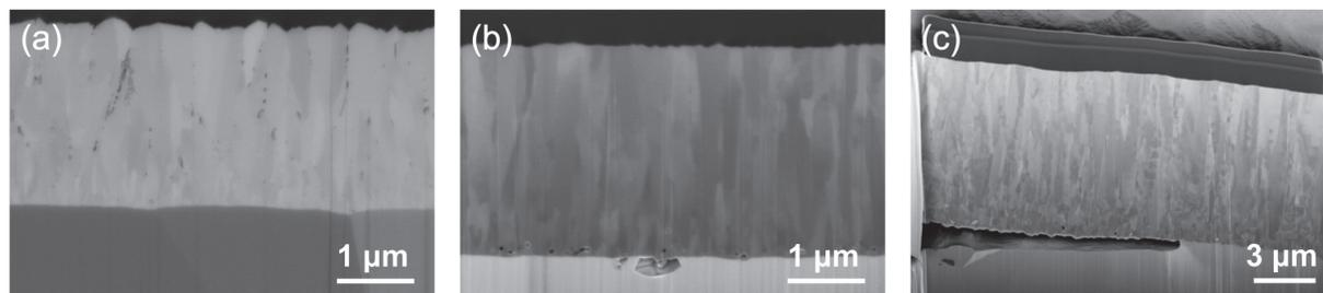
Figure 1: FIB-SEM images of (a) a porous film; (b) a film with voids at the interface; (c) a partially delaminated film.
