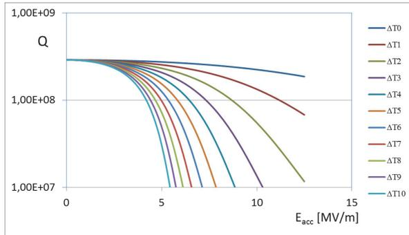
Figure 3a: Q-factor vs accelerating field for a thin film Nb/Cu 6GHz cavity at  $T=1.8\text{K}$ , after 10 interactions. The parameter used for calculation were  $R_0=0.8\mu\Omega$ ;  $R_B=6\text{cm}^2\text{K}/\text{W}$ ;  $A=6\text{e}-3\Omega$ ;  $\Delta_0/K_B=17,5\text{K}$ ;
