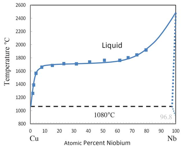
Figure 2: The Cu-Nb phase diagram, after D.J. Chakrabarti and D.E. Laughlin [15].
