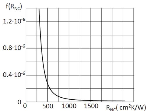
Figure 5: Distribution function  $f(R_{Nb/Cu})$  got by inverting Eq. 9 using as input data the  $Q$ - $E_{acc}$  data reported in Fig. 4.
