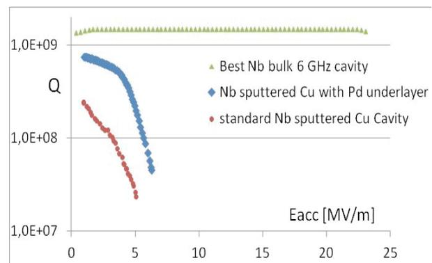
Figure 6: -  $Q$  vs  $E_{acc}$  at 6 GHz, for a standard Nb sputtered Cu cavity (red circles), for a sputtered Cavity with a Pd underlayer, and for comparison the best result obtained for bulk Nb at 6 GHz.
