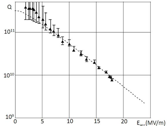
Figure 4: Q-factor vs  $E_{acc}$  for a thin film Nb/Cu 1.5GHz cavity at  $T=1.7\text{K}$  realized at CERN [4]. The data are the experimental points of the highest curve in Fig. 2 for  $E_{acc}>2\text{MV}/\text{m}$ . The dashed line represents the data fitting using the distribution function  $f(R_{\text{Nb}/\text{Cu}})$  in Fig. 5.
