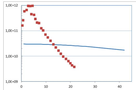
Figure 1: Typical behaviour of  $Q$ -factor versus the accelerating field for bulk Niobium cavities compared to Nb film sputtered cavities. The  $Q$  factor displayed by red squares is referred to a 1.5 GHz Nb Sputtered Cu cavity measured at 1.7 K [4]. The  $Q$  factor displayed by the blue line, is referred to 1.3 GHz bulk Niobium cavities measured at 1.8 K.
