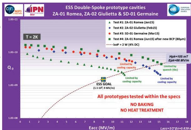
Figure 6: Q-curves vs. Eacc of the 3 cavities.
