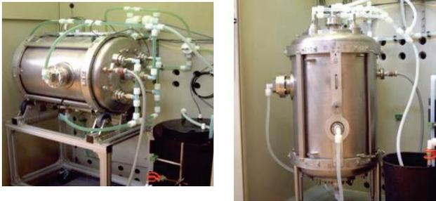
Figure 5: BCP set-up: horizontal (left) and vertical (right).
