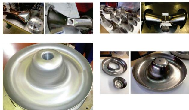
Figure 4: Spoke bar and end-cup fabrication from E. Zanon (left) and SDMS (right).
