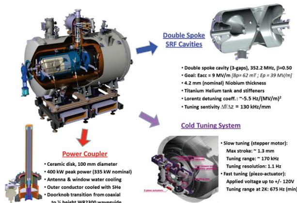
Figure 2: 3D model of the prototype cryomodule and the main components.
