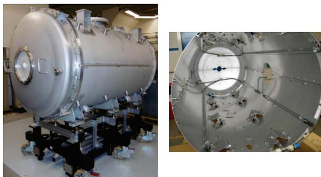
Figure 3: Vacuum vessel set on its mechanical support (left) and the thermal shield (right).
