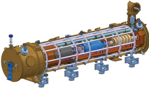
Figure 11: Cryomodule cross section.
