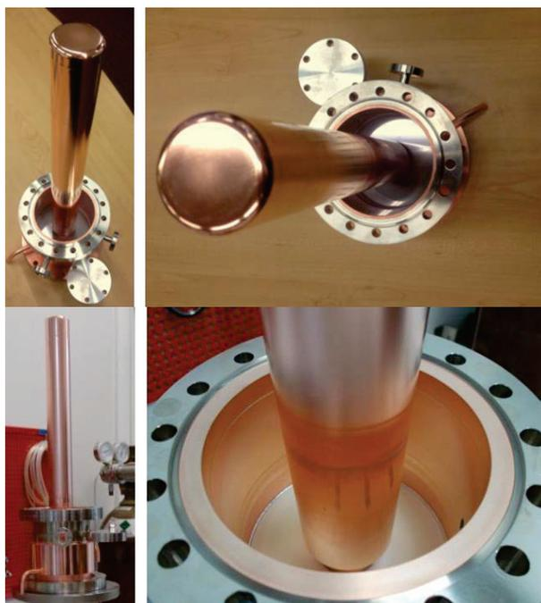
Figure 9: Prototype couplers from SCT (upper) and PBM (lower).
