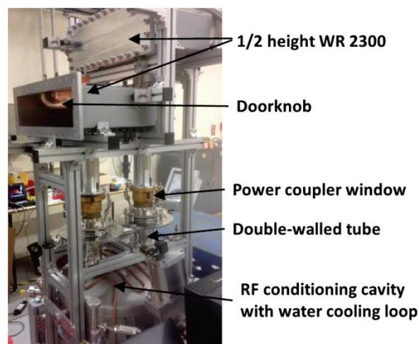
Figure 10: RF conditioning test bench.
