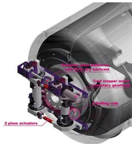
Figure 7: 3D model of the Cold Tuning System for spoke cavities.
