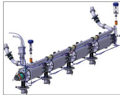
Figure 12: The cavity string equipped with the cryogenic pipes.
