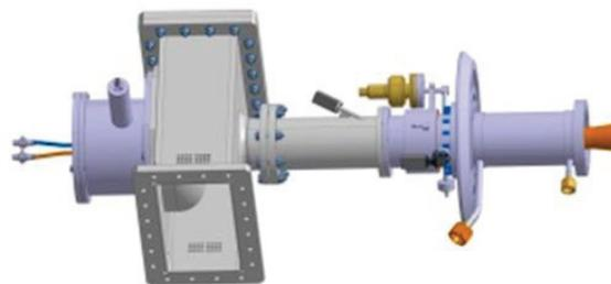
Figure 15: 3D model of the power coupler.
