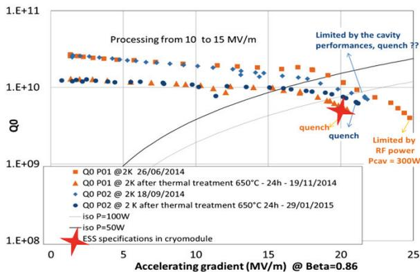
Figure 13: Q-curves of the two high beta prototype cavities before and after heat treatment for hydrogen degassing.
