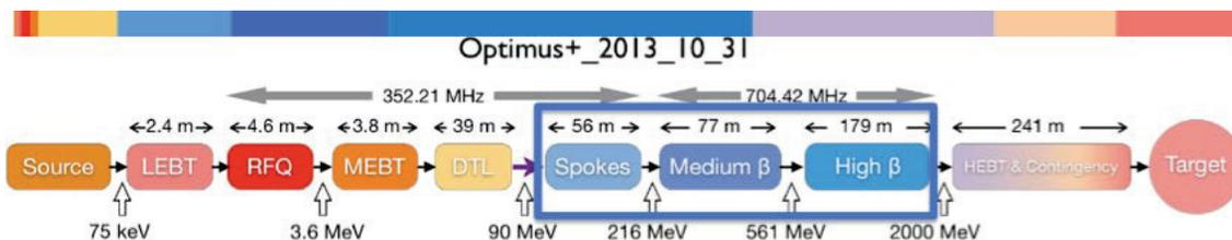
Figure 1: Block diagram of the ESS linear accelerator.
