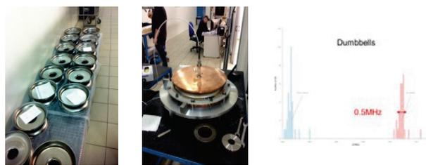
Figure 14: Dumbbells of the medium beta cavities prototype (left) and frequency measurements (right).
