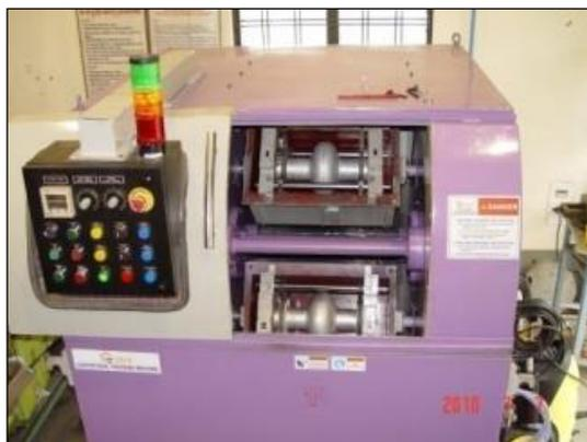
Figure 7: Centrifugal barrel polishing (CBP) machine.
