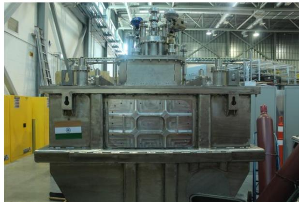
Figure 11: Injector Cryo Module at TRIUMF for the VECC superconducting Electron Linac (e-Linac).
