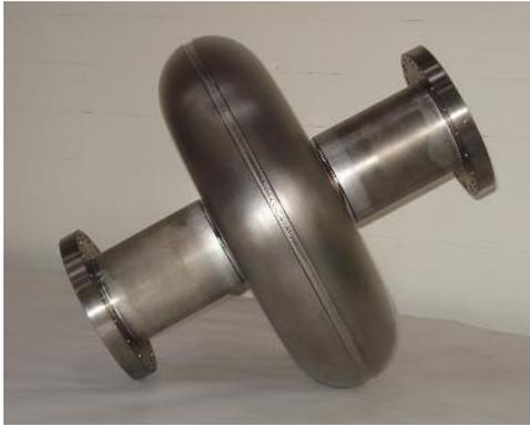
Figure 12: Single cell 650 MHz,  $\beta=0.6$  niobium cavity developed by VECC and IUAC.
