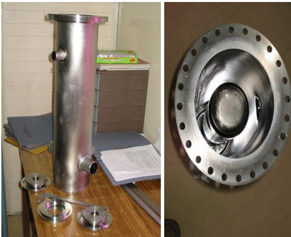
Figure 1: The indigenous niobium QWR successfully fabricated and tested at IUAC.
