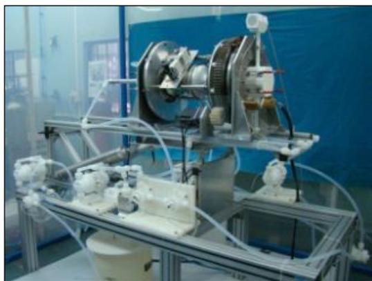
Figure 8: Electro-polishing setup.
