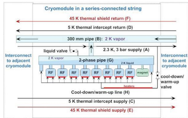
Figure 7: Scheme of cryogenic flow in the module.
