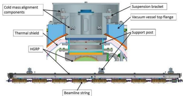
Figure 5: Cold mass support and alignment system.
