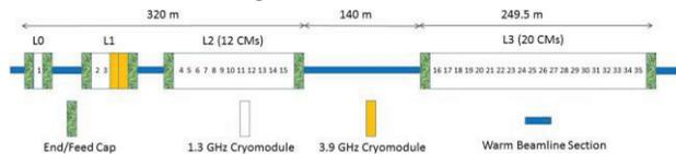
Figure 1: LCLS-II Linac with cryomodules in sections.
