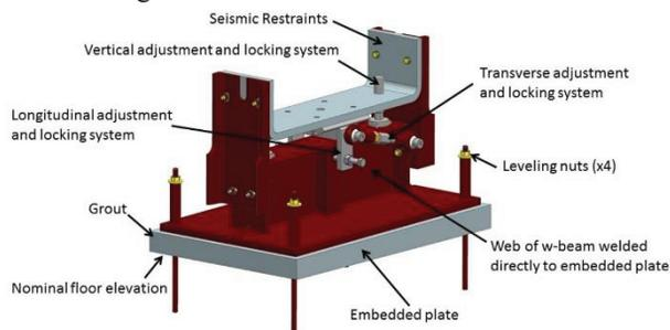
Figure 12: Cryomodule adjustable support stand and its attachment to the tunnel floor.
