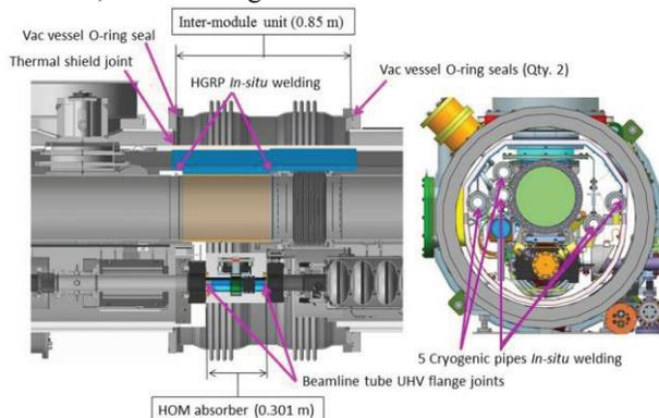
Figure 11: Cross-sectional views showing inter-module connections.
