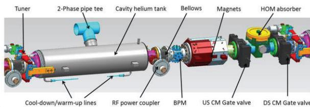
Figure 4: Components in dressed RF cavity and beamline string.
