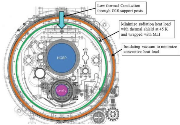
Figure 10: Cryomodule thermal insulation.
