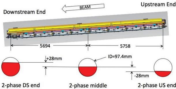
Figure 9: Liquid helium levels in the 2-phase pipe with 0.5% SLAC tunnel slope, with pipe sized to accommodate liquid levels both downstream and upstream.
