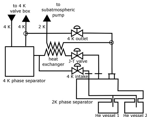
Figure 6: Basic principle of the integrated 4 K/2 K Joule-Thomson expansion.
