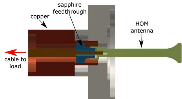
Figure 5: HOM antenna (green) and feedthrough (blue) based on Kyocera design. Sapphire feedthrough was chosen for a better thermal conductivity.
