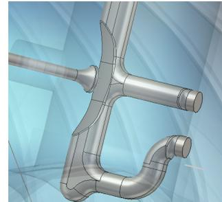
Figure 4: Assembly of the f-part and HOM antenna. The cavities and HOM coupler container are shown in transparent blue. F-part designed by DESY [16].
