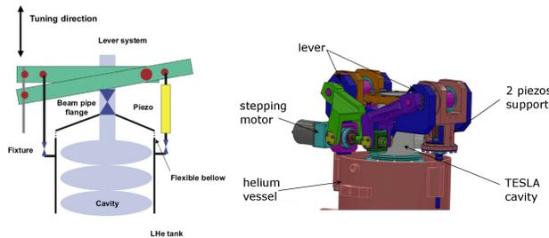
Figure 3: XFEL/Saclay tuner.
