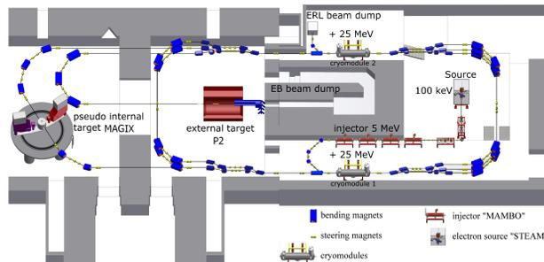
Figure 1: Possible configuration of the MESA design. The beam pipe is allocated around an existing beam dump which will be used in external beam (EB) mode.
