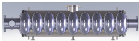
Figure 3: The e-Linac nine cell cavity with jacket.
