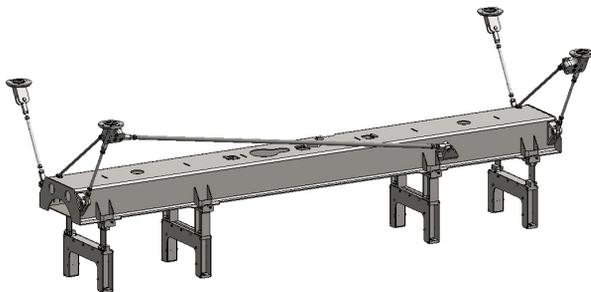
Figure 4: Strut and strong-back assembly.
