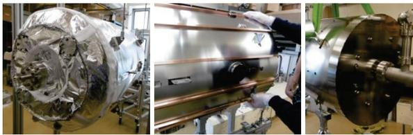
Figure 2: Left: MLI on the cavity. Centre and right: actively cooled magnetic shield.
