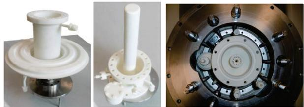
Figure 5: 3D mock-up of the coupler mounted on the vacuum vessel interface.
